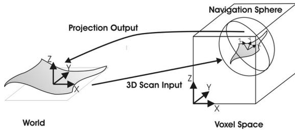
**Figure 7. Transformation between world and voxel coordinate systems**
